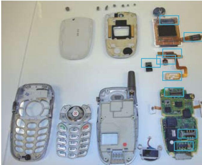
Disassembled Phone – Connectors Highlighted
