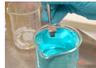
Test procedure calls for a one-minute dip in copper chloride solution.
