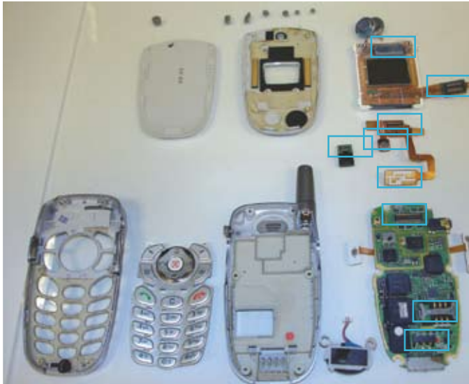
Disassembled Phone – Connectors Highlighted
